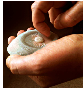
Figure 1. Finger rubbing a rough surface. Vibrations generated by the finger rubbing against the textured surface are sensed by a piezo-microphone
