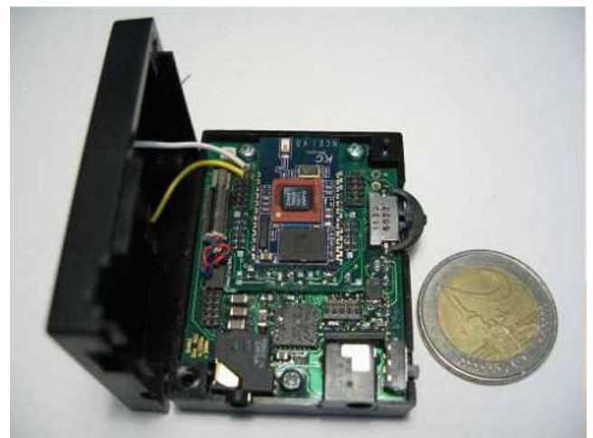
Figure 8: The SHAKE sensor. This is complete inertial sensing platform running over Bluetooth.
