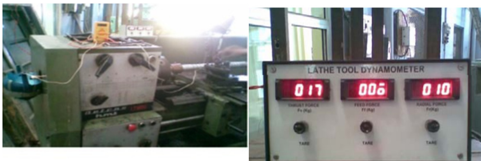
Figure 3: Experimental set-up of HMT heavy-duty lathe with a tool dynamometer.
