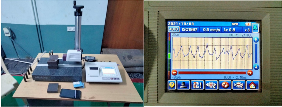
Figure 4: SURFTEST SJ-410 surface roughness tester.
