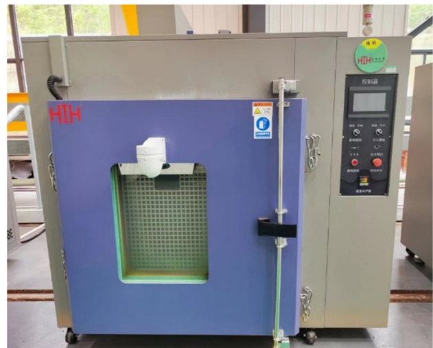
Figure 2: High-temperature test oven for rubber aging.
