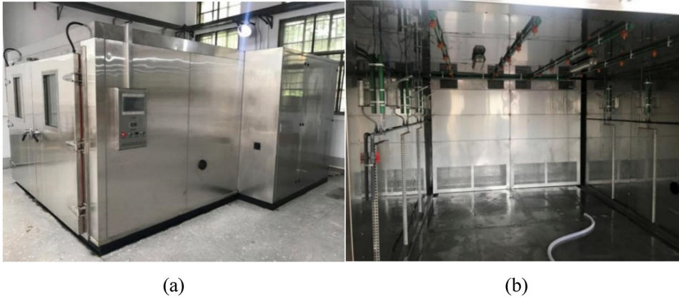
Figure 2: Environmental simulation test chamber: (a) appearance of the test chamber and (b) inside of the test chamber.
