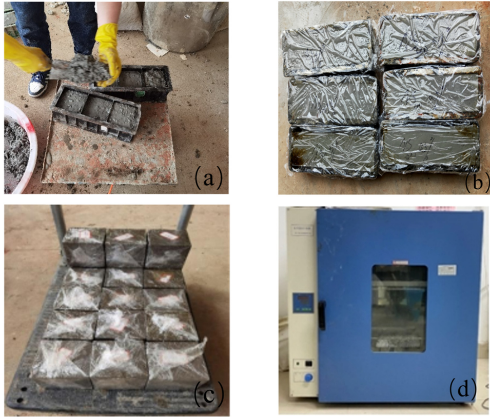
Figure 3: Sample preparation and curing: (a) pouring and vibrating, (b) solidification, (c) demolding, and (d) high-temperature curing.
