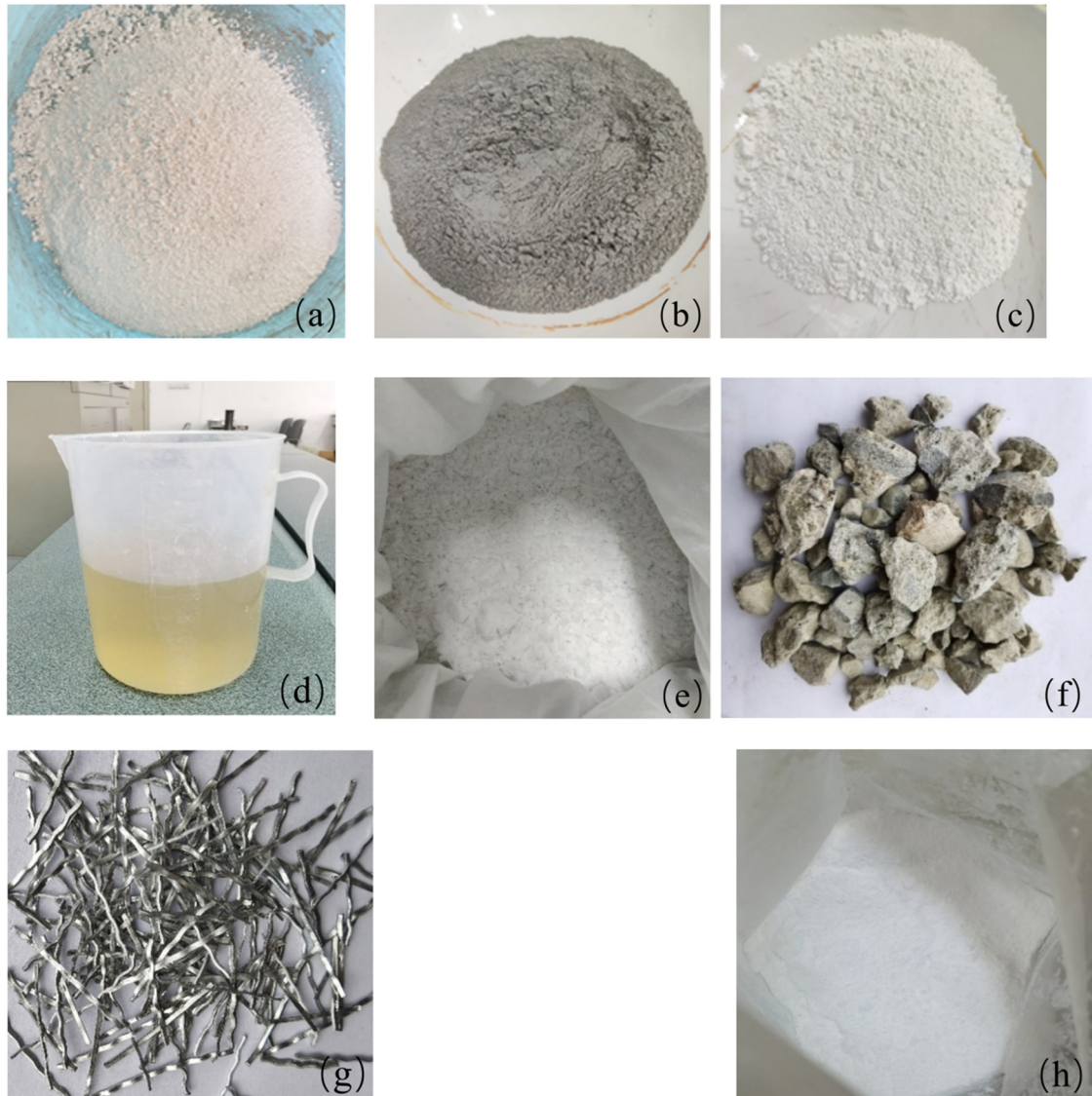
Figure 1: Experimental materials: (a) CG, (b) FA, (c) slag, (d) sodium silicate, (e) NaOH, (f) RCA, (g) SF, and (h) NA.
