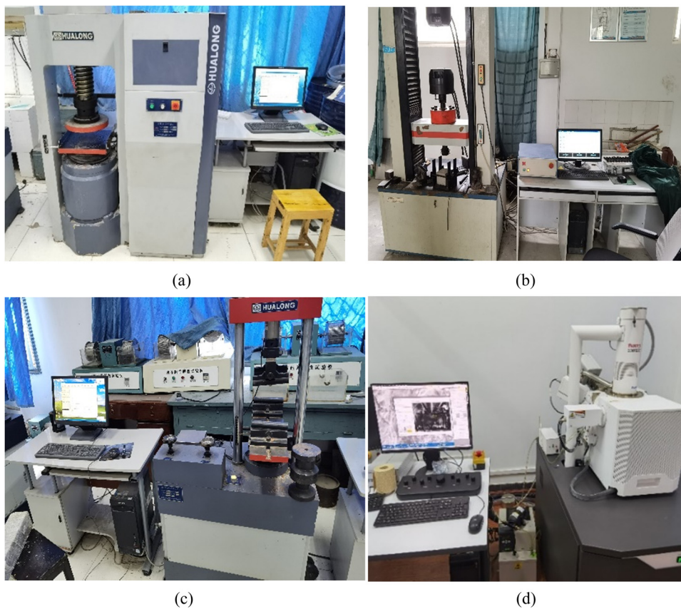
Figure 4: Laboratory apparatus. (a) Machine for compressive test, (b) machine for splitting tensile test, (c) machine for flexural test, and (d) SEM.
