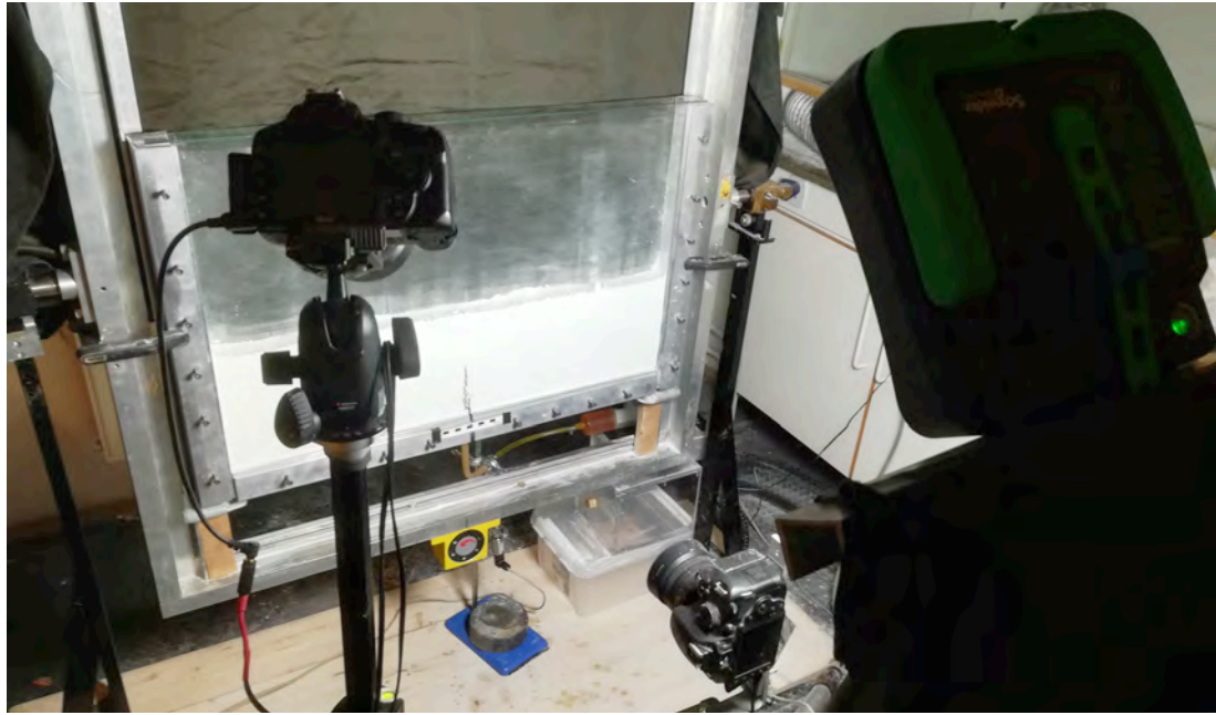
Figure 8. The 2D Hele-Shaw setup filled with compacted cohesive fine-grained host. The intruding fluid is golden syrup injected at constant flow. Fine-grained aluminium silicate has been introduced into the host such that it is possible to apply Digital Image Correlation to study small deformations.
