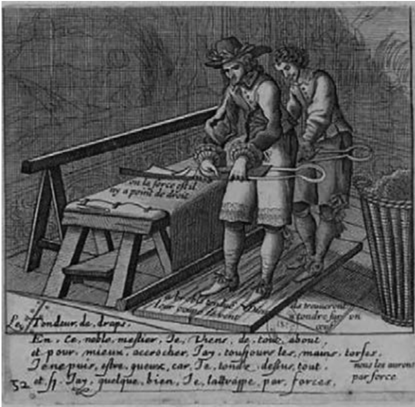
Figure 1.4 Cloth shearers working with a crook or mailloche in their right hands. Engraving, France, seventeenth century
