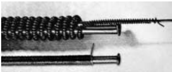
Figure 5: Coiled-coil (top, 1933) and simple coil (bottom, 1913) filaments. ([1])
