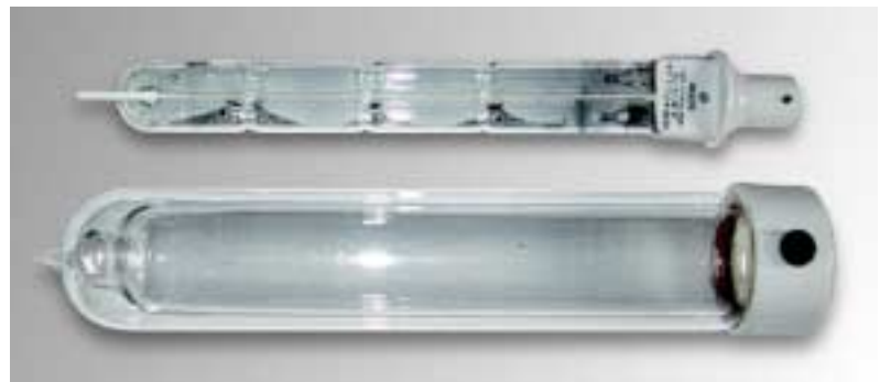
Figure 22: Sodium lamp with bamboo-shaped discharge tube and detachable Dewar outer jacket. (Philips SO/H60W, 1955)
