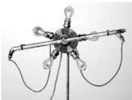
Figure 17: Cooper-Hewitt tube connected in series with carbon filament lamps, which act as a ballast. (ca. 1910, [8])
