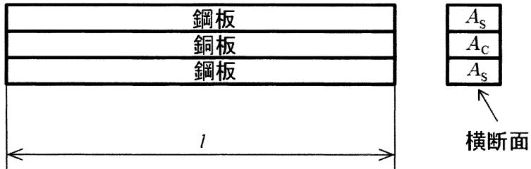
$$\textcircled{1} \quad \sigma_s = \frac{(\alpha_c - \alpha_s)E_c E_s A_c}{(2E_s A_s + E_c A_c)} \Delta T, \quad \sigma_c = -\frac{2(\alpha_c - \alpha_s)E_c E_s A_s}{(2E_s A_s + E_c A_c)} \Delta T$$
