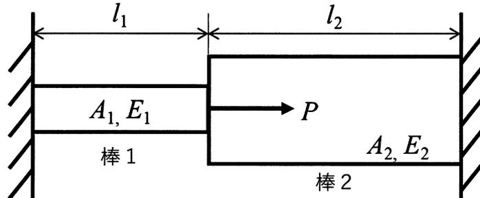
①  $\sigma_1 = \frac{E_1 l_1}{A_1 E_1 l_2 + A_2 E_2 l_1} P, \quad \sigma_2 = -\frac{E_2 l_2}{A_1 E_1 l_2 + A_2 E_2 l_1} P$
