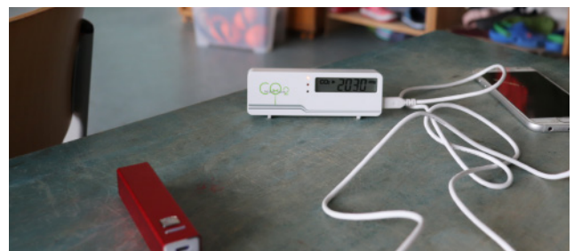
► A mini CO 2 monitor was used which contains a traffic light system for classifying the indoor CO 2 concentration. | © HEAL |
