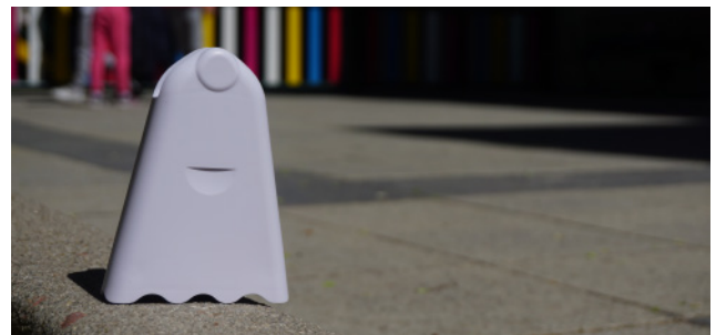
► The low cost air monitor works with a light scattering method to measure fine particulate matter. | © AEEA |
