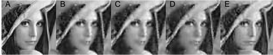
Figure 1: Different reconstruction of Lena for a given file size of 2000 bytes. (A) Detail of the original 128x128 image; reconstruction using (B) MP; (C) MP with Look-Up-Table; (D) Weighted MP; and in comparison with (E) JPEG (Quality 32)
