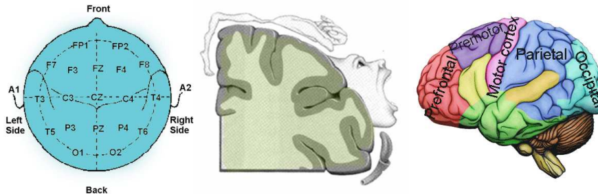
Fig. 2: Left The placement (and names) of the electrodes on the head according to the 10-20 international system. Middle The homunculus shows the mapping of the different body parts to the motor cortex. Notice that the hands occupy a large region. Right The different lobes of the brain. The motor cortex corresponds to the picture in the centre.
