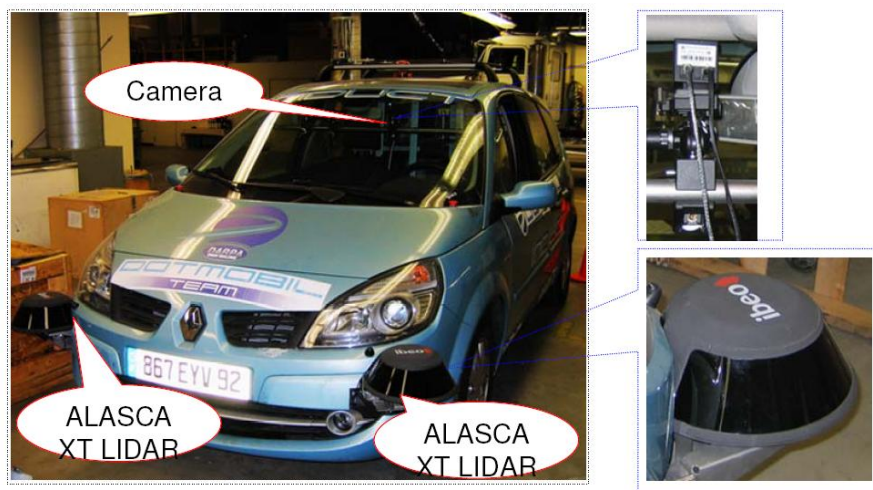
Figure 1-1. The mobile sensing platform. This probe vehicle carries one camera and two IBEO ALASCA XT LIDAR sensors.
