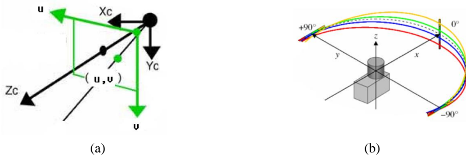
Figure 3-2. Two coordinate systems. (a) The camera coordinates and screen coordinate systems, and (b) the LIDAR coordinate system.
