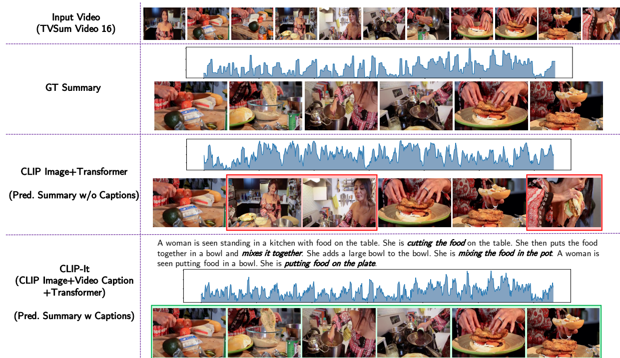
Figure 3.3: Comparison of ground-truth summary to results from CLIP-Image+Transformer and the full CLIP-It model (CLIP-Image+Video Caption+Transformer). The input is a recipe video. Without captions, the model assigns high scores to certain irrelevant frames such as scenes of the woman talking or eating which hurts the precision. With captions, the cross-attention mechanism ensures that frames with important actions and objects are assigned high scores.
