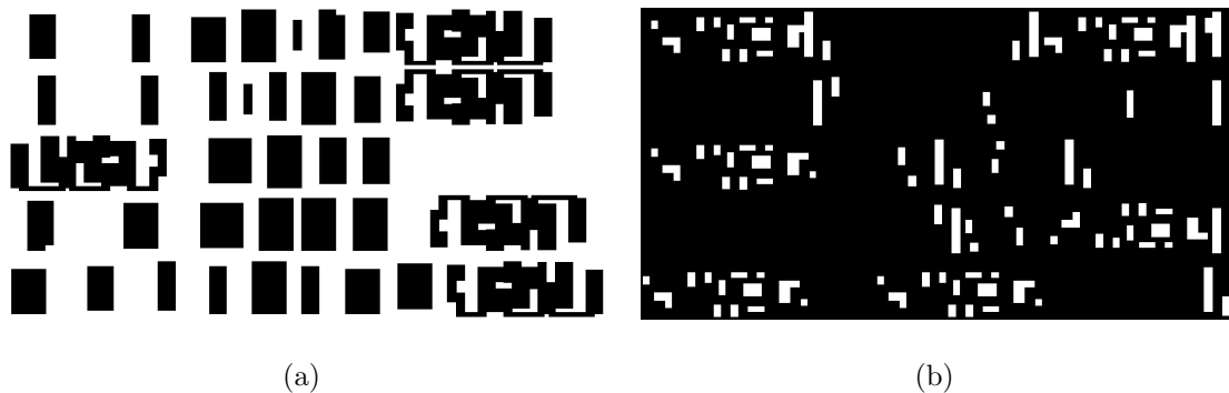
Figure 4.10: Trim-mask layout snippet for poly-lines (a) and contacts (b). In (a), simple large blocks correspond to cells with unidirectional poly-lines and more complex shapes correspond to flip-flops with bidirectional poly-routing. In (b), both flip-flop and combinational logic regions have simple trim-mask features.
