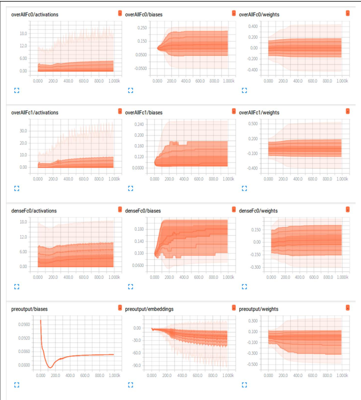
Figure 39 Cluster plot of the weight distribution, bias distribution, and activation distribution changes in dense-sparse model over time. Y-axis represents the parameter value, and the X-axis represents the training iteration (training time). Darker color represents more parameters falling within the darker area. The parameters are spreading out during training.
