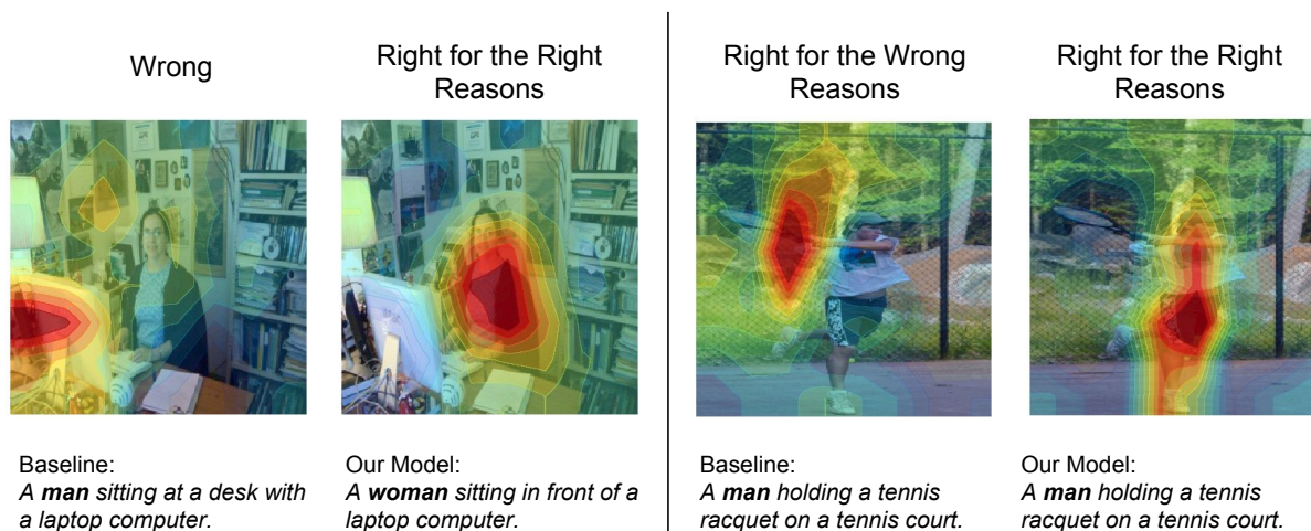
Figure 4.1: Examples where our proposed model (Equalizer) corrects bias in image captions. The overlaid heatmap indicates which image regions are most important for predicting the gender word. On the left, the baseline predicts gender incorrectly, presumably because it looks at the laptop (not the person). On the right, the baseline predicts the gender correctly but it does not look at the person when predicting gender and is thus not acceptable. In contrast, our model predicts the correct gender word and correctly considers the person when predicting gender.
