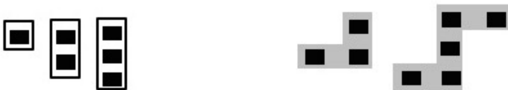
(a) Examples of DSA groups allowed in both 193i and EUV (b) Examples of DSA groups allowed in EUV but not in 193i
