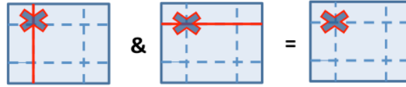
Figure 3.5: Checking conflicts between routing options of different nets by ANDing Node Representations
