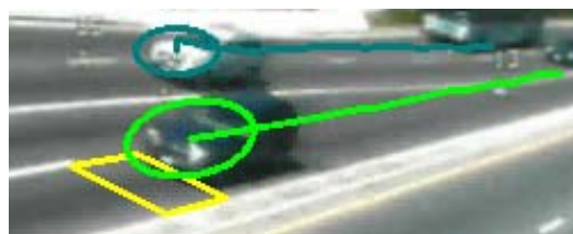
Figure 4-5: Virtual loop is triggered when a vehicle reaches it
