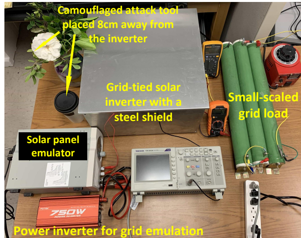
Figure 2.6: A scaled-down testbed of a power grid.
