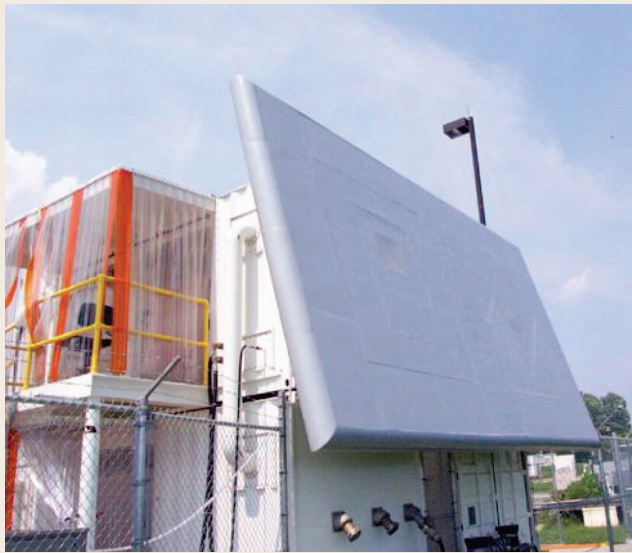
[FIG3] (a) Representation of the waveform-agile tracking algorithm that selects waveform parameters A, B, and the phase function by minimizing the predicted MSE. (b) Naval Research Laboratory (NRL) radar on Chesapeake Bay for testing waveform-agile sensing applications [55].
