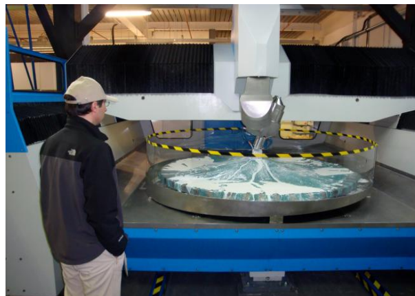
Figure 3.85. Large-scale Zeeko polishing machine at Optic Glyndwr.
