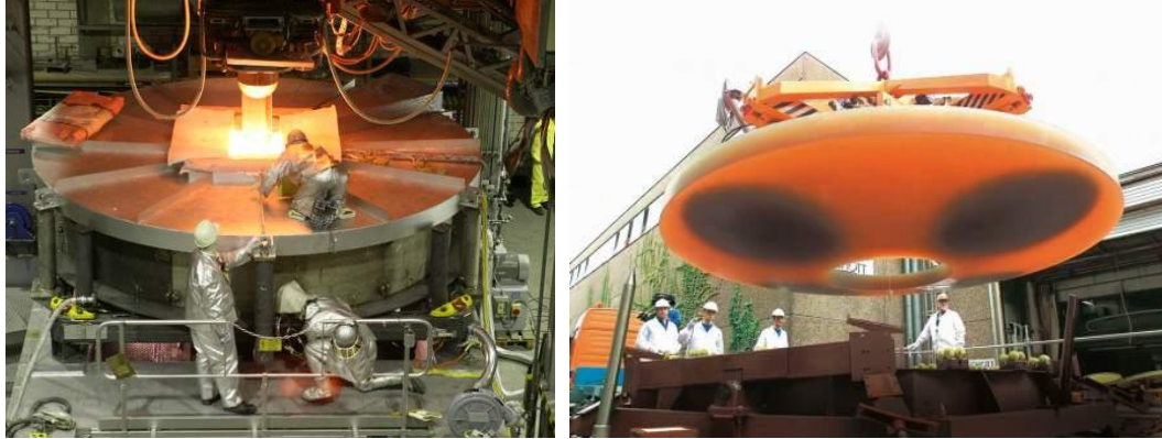
Figure 3.121. Schott 4-metre blank. Left: Casting. Right: Finished product (Courtesy Schott).
