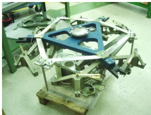
Figure 3.116. Components of the CESA design for the segment support and prototype system.
