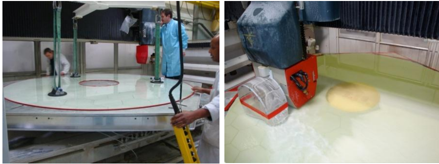
Figure 3.155. The 2.7-metre 2 mm thin shell on the blocking body and in the thinning process.
