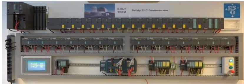
Figure 3.193. The scale-one demonstrator of the interlock and safety system.
