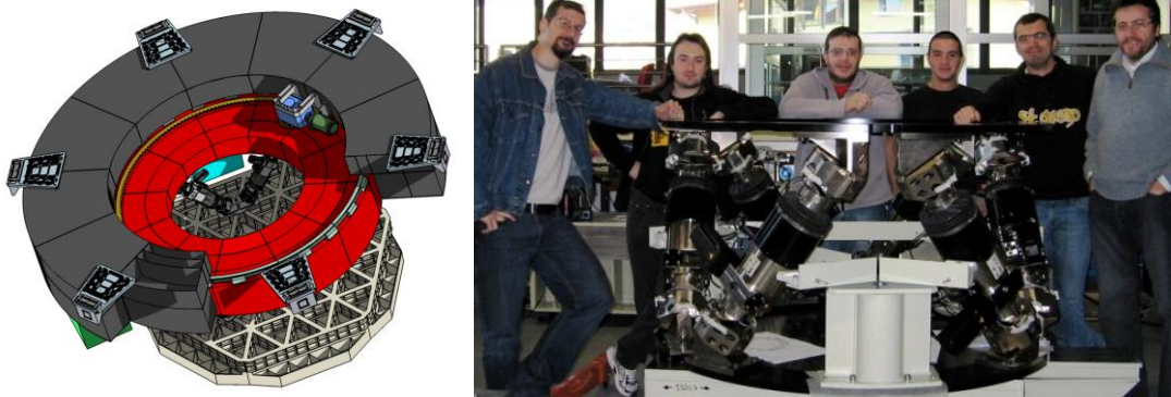
Figure 3.152. M4 mounting structure and positioning system for the Dark Energy CAMera.
