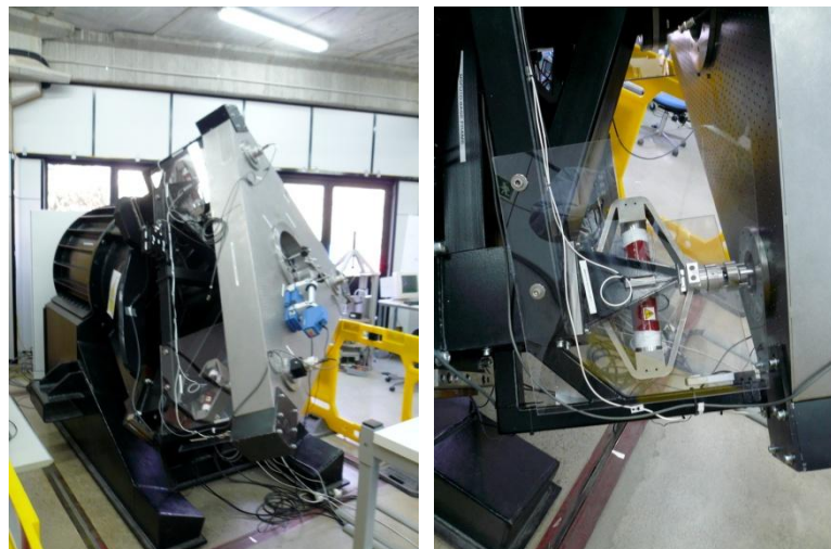
Figure 3.167. Prototype scale-one unit with dummy mirror and one of three actuators mounted in prototype unit.
