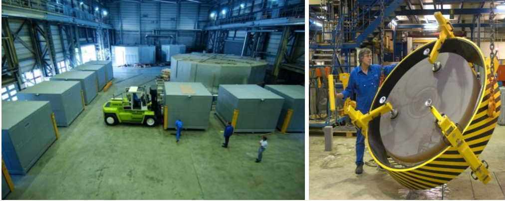
Figure 3.82. Left: Annealing facility at Schott in Mainz. Right: Sample boule.
