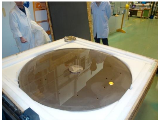
Figure 3.115. ULE polished segment before cutting at Sagem.
