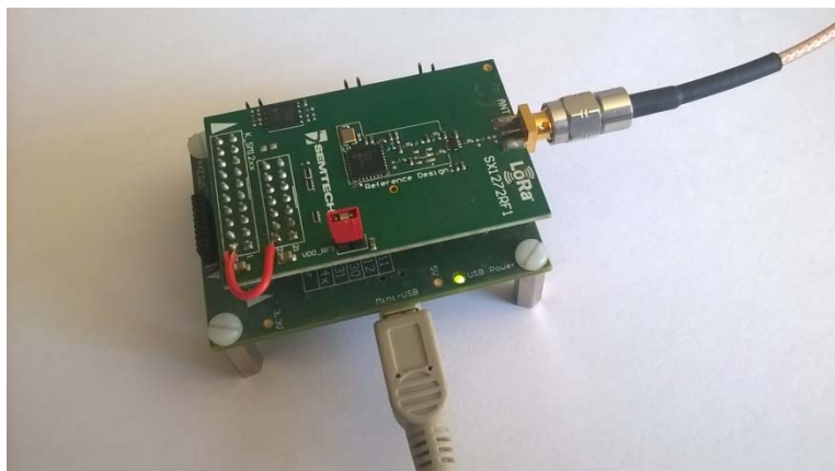
Figure B.2: FSK receiver
