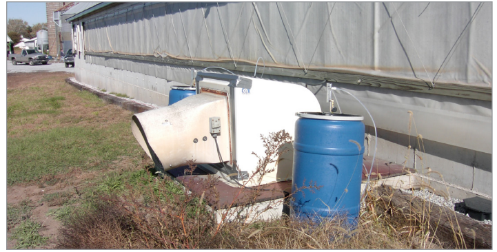
Figure 2. Odor air sampling at a pit fan in the field study of an additive at finishing swine barns.
