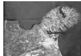
PALSAR-1 FBD mode, processed over Christchurch New Zealand, with RFI filtering. SAR raw data courtesy of NASDA, Japan.
