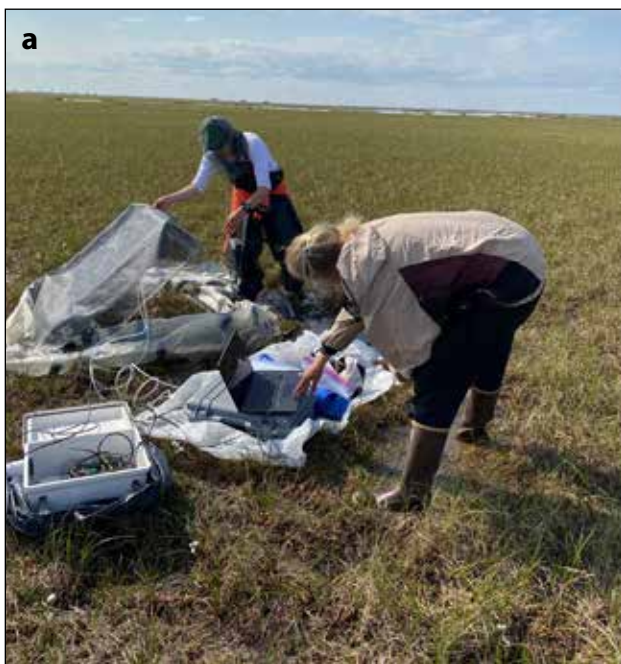
Figure 36. Trace-gas flux measurements. a. Anja Kade and Josephine Mahoney preparing to make flux measurements using a 0.7-m x 0.7-m chamber. b. Anja Kade recording trace-gas flux and respiration in a wet-tundra plant community. (Photos: J.L. Peirce, IMG 4212, IMG 4197)
