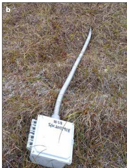
Figure 39. Typical setups of loggers. a. A station in a flood prone wet/ aquatic-tundra location where the logger is elevated on a tripod. b. Station located in moist-tundra site, where the logger case is located on the ground. (Photos: N. Hasson)
