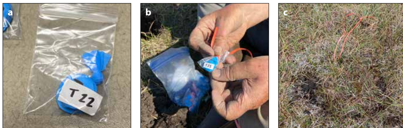
Figure 32. Temperature logger placement in terrestrial plots. a. Sealed logger placed in small zip-top bag labeled with the plot number. b. Orange ribbon attached to the bag. c. Soil pit after insertion of the loggers just beneath the surface and at the base of the organic layer, with orange ribbons displayed above ground. (Photos: J.L. Peirce, IMG 4510, IMG 4632, IMG 4823).
