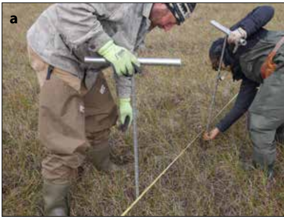
Figure 11. Thaw-depth measurements. a. Measuring thaw along 40-m transect at BP-1. (Photo: H. Bergstedt, P1060163). b. Thaw depths (means \pm standard deviations) for the transects sampled 15–17 August 2020.
