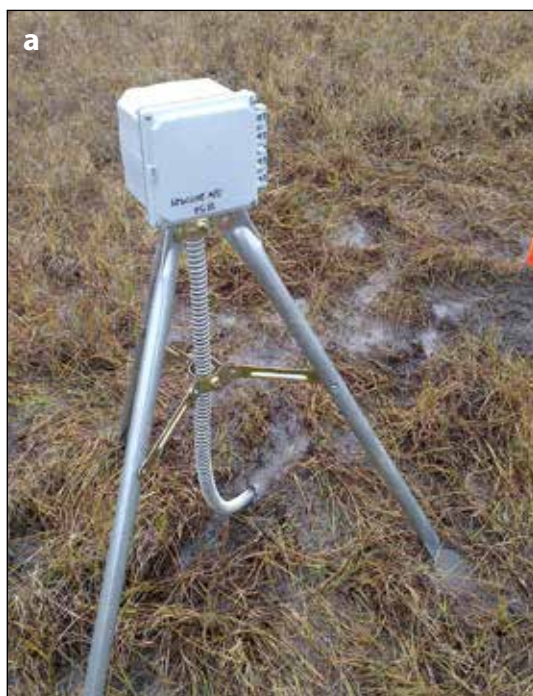
Figure 39. Typical setups of loggers. a. A station in a flood prone wet/ aquatic-tundra location where the logger is elevated on a tripod. b. Station located in moist-tundra site, where the logger case is located on the ground. (Photos: N. Hasson)
