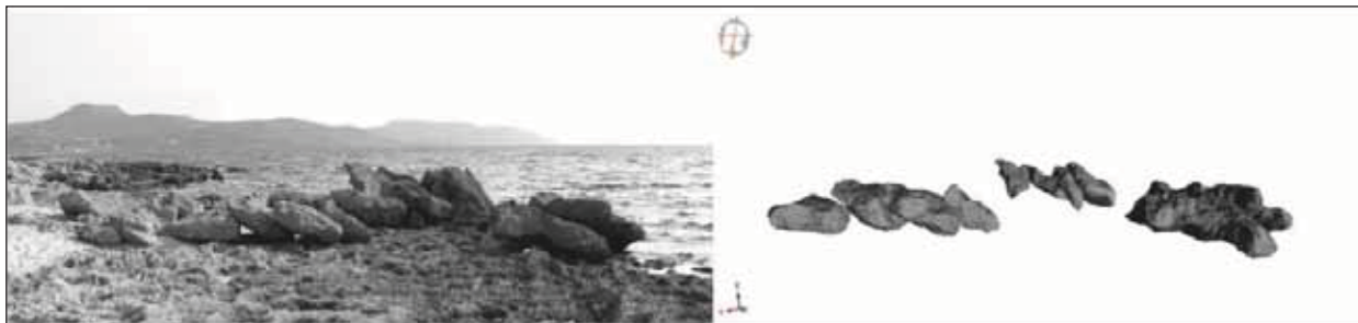
Fig. 4: Picture and 3D-model of a blocktrain near Cape Skalas (SE-Lakonia) modeled by the software RiScanPro. The biggest measured block has a maximum weight of about 4.6 t. In the background Elaphonisos Island with its uplifted marine terraces is visible (photo taken by K. Ntageretzis, 2008, model of dislocated boulders by D. Hoffmeister, 2009).
