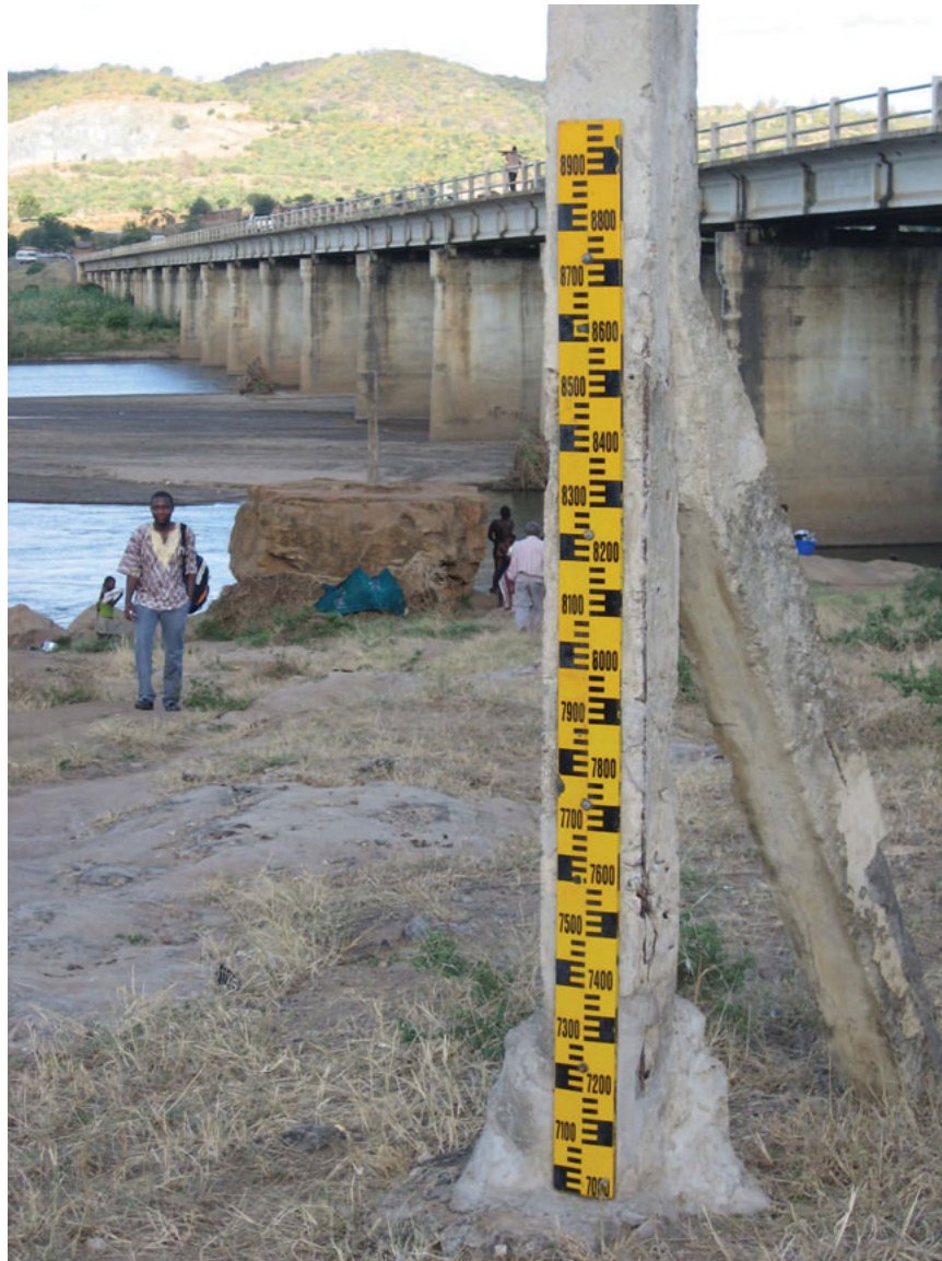
Staff gauge at the Chingozze Station on the Revuboe River, Mozambique. Source: D. Kull, 2012.
