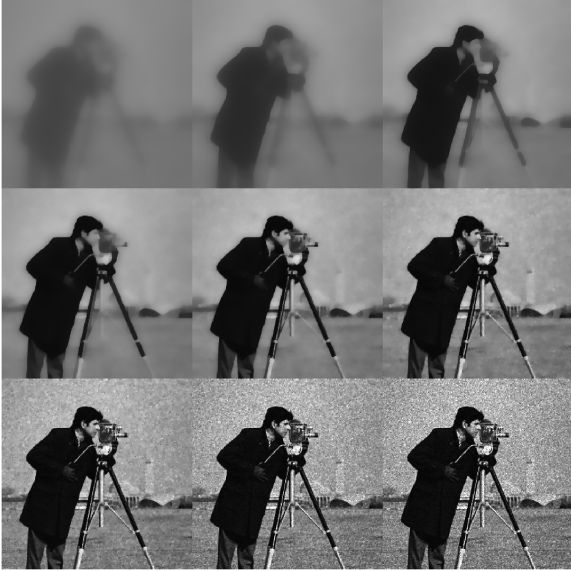
Figure 4: Multiscales x_k for k = 4, 5, \dots, 12 in the SO MHDМ recovery of the cameraman image. In this example, our proposed stopping index k^*(\delta) = 9 = k_{min} is optimal (Refer to the diamond-labeled curves in Fig. 6).
