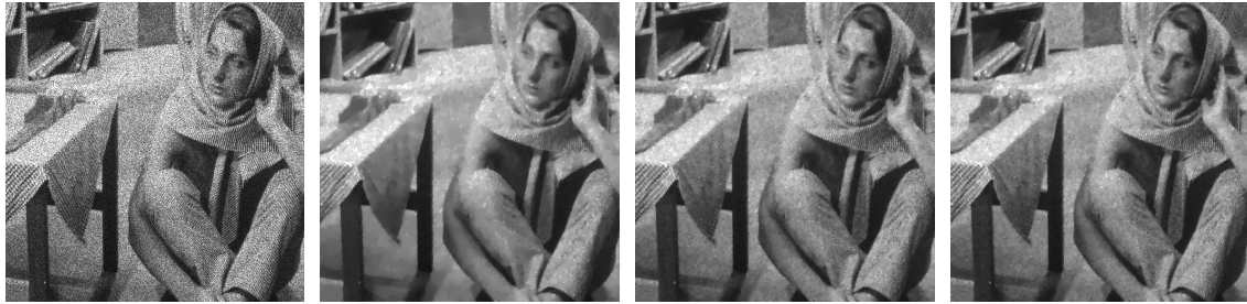
Figure 17: Recoveries from high noise (standard deviation 0.32). From left to right: noisy image ( RMSE = 41.25 , SNR = 10.00 ), DZ model ( RMSE = 17.5233 , SNR = 17.44 , \lambda = 0.08 ), the SO MHDHDM tight ( k_{min} = 6 , RMSE = 16.37 , SNR = 18.03 ) and AA-log MHDHDM tight recoveries ( k_{min} = 6 , RMSE = 16.38 , SNR = 18.02 ).
