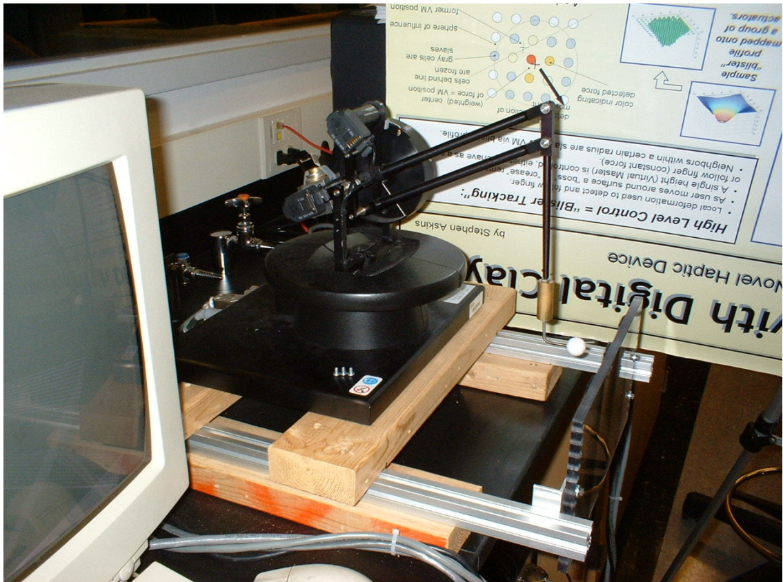
Figure 6.2: Human Experiment Setup Slave Side with Mount for Surface Contour and Maze Blocks
