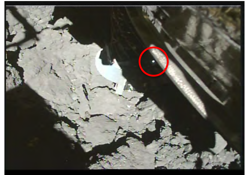
Laser light from the LRF-S2 imaged by CAM-H (At the 2 nd touchdown)
