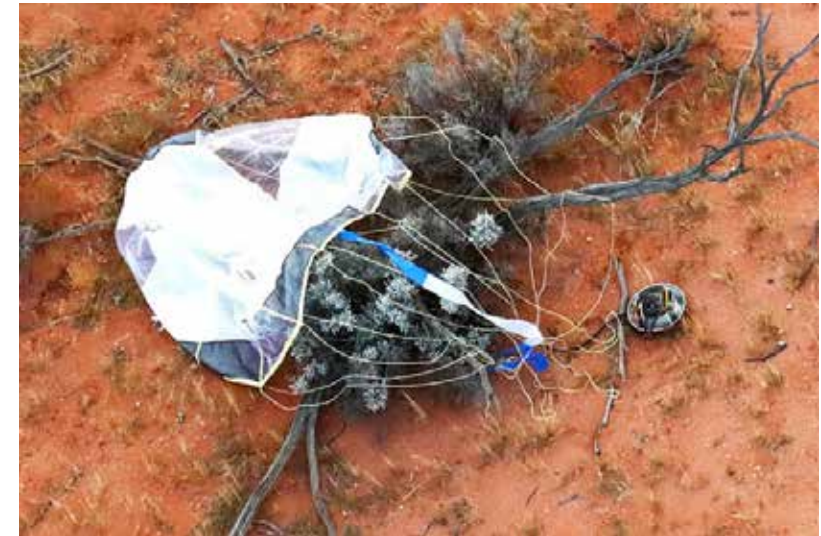
Capsule and parachute as found in the Woomera desert, Australia.
