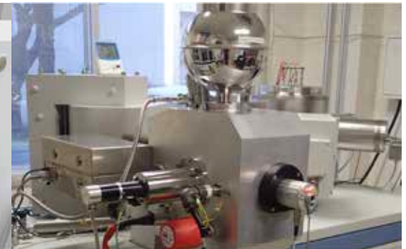
Thermal ionization mass spectrometer for isotope analysis and dating (© Tokyo Institute of Technology)
