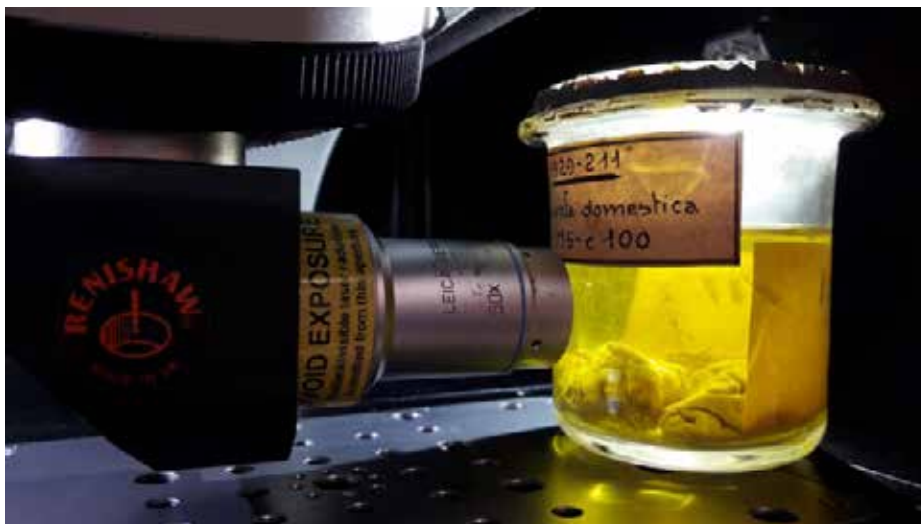
Figure 1. Identification of a fluid through the jar thanks to Raman microspectroscopy (piece of the MNHN comparative anatomy fluid collection: brain of Sus scrofa domestica in Bouin's solution – inventory number MNHN-ZM-AC-1929-211). © CRC-MNHN - S. Cersoy
