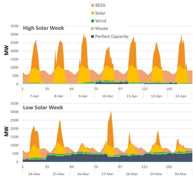
Figure 2. Representative high and low solar weeks and the need for firm renewables.
