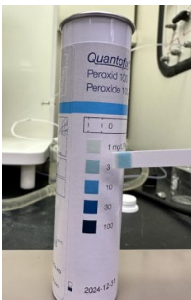
Figure 3. Colorimetric test strip indicating the positive detection of hydrogen peroxide after insertion into the bulk solution (post-production test).
