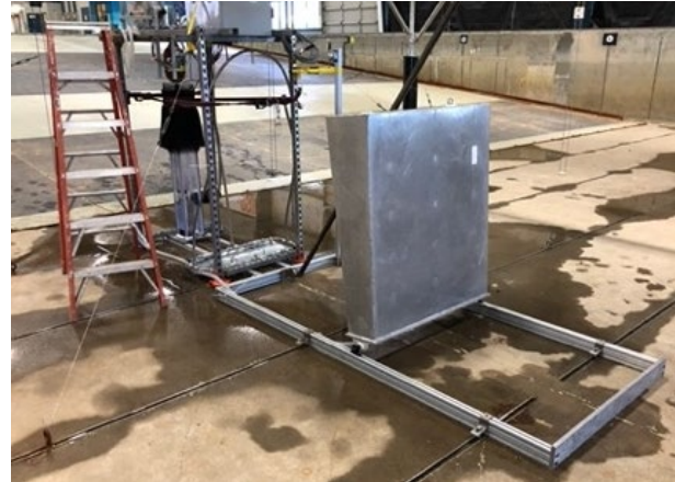
Figure 1. HNEI's HAWSEC system in Oregon State University's wave basin for testing.
