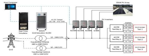
Figure 1. HNEI GridSTART's Advanced Power System Lab architecture.
