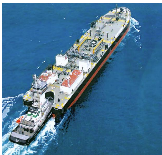
Figure 45: The Brandywine: An Oil-Products ATB (courtesy Argent Marine)
