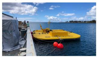
2. Deployment of the C-Power SeaRay WEC. This is a stand-alone (not grid-connected) deployment of a small, 1kW device that will feed power to a subsea acoustic sensing system from Biosonics, as well as other environmental sensors. The device was deployed at WETS in early October 2023, but suffered some early damage and will need to be redeployed at a future date.
