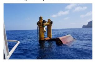
Oct 2018 to Mar 2019: HNEI led effort to redeploy Lifesaver at 30m with modifications to moorings and integration of UW sensor package and subsea charging capability, which drew its power from the WEC itself. This use of wave energy to power an offshore sensing suite was an important national first.
