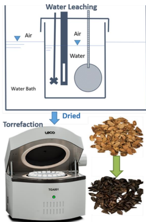
Figure 12. Laboratory scale leaching and torrefaction test equipment.
