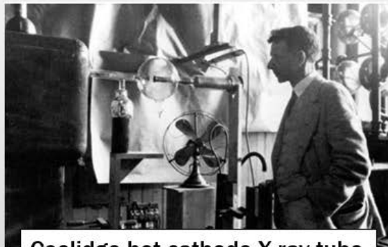
Coolidge hot cathode X-ray tube
