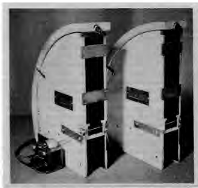
Figure 6. Film cassette with tube and rotating device.
