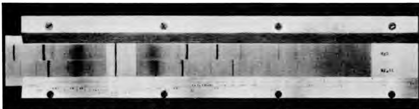
Figure 1. X-ray powder diffraction patterns in calibrated scale. MoK \alpha radiation.
