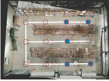
Figure 3: The warehouse environment with topological map overlaid. Blue circles show initial robot locations.
