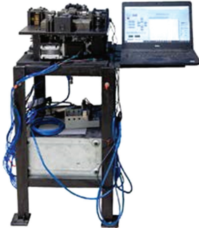
The photograph of an indigenously developed in-situ multiaxial universal testing equipment
