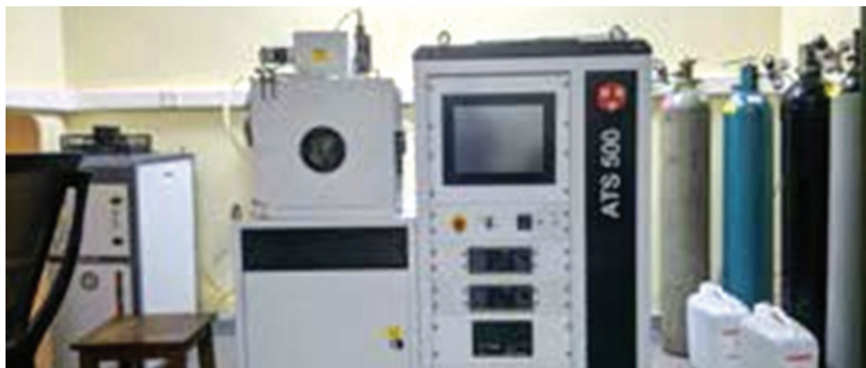
Photograph of the magnetron sputtering unit installed in the department in 2020-2021
