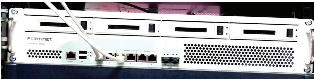
Web Application Firewall: WAF Fortinet 1000 series Acts as the firewall for websites
