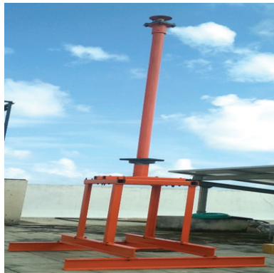
Figure 3: Final assembly of Savonius turbine
