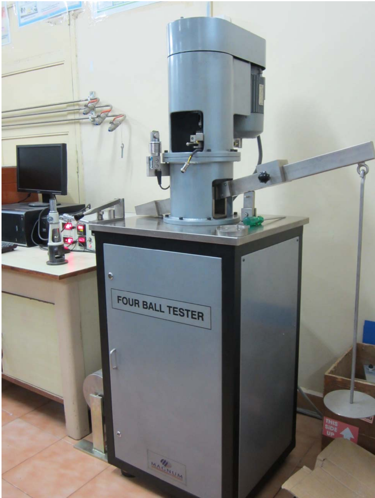
Fig. 2 (New) Facility for evaluating frictional characteristics of nanolubricants
