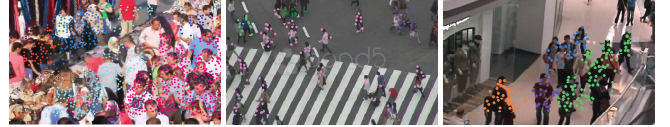
Figure 3: Group detection using coherent filtering [Zhou et al. , 2012a], in which different groups are indicated with different colors (best viewed in color version).
