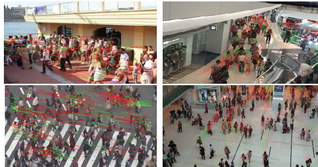
Figure 7: Prediction of future paths with coherent regularization, in which the red paths are reliable tracklets obtained from KLT trackers and the green ones are the forecasted paths from the cLSTM.
