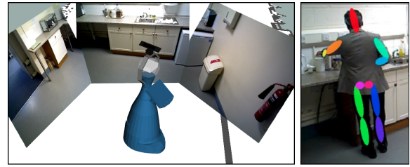
Figure 1: (left) Mobile Scitos A5 robot gathering RGB-D data. (right) An example of a human pose estimate.
