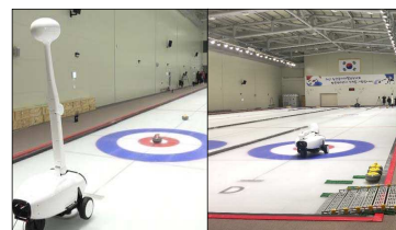
Figure 1: The AI curling robots play the curling game on a real curling ice sheet. (Left) The skip robot recognizes the game state using the location of stones. (Right) The thrower robot is throwing in order to deliver the stone to the target location chosen by the AI strategy engine. https://youtu.be/yXygf8oz58k
