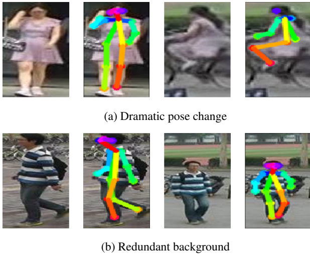
Figure 2: The examples of various poses in the re-ID scenes, where each row shows the different poses of one person. The original images are shown in the first and third columns. The pose information obtained by our model are shown in the second and fourth columns.
